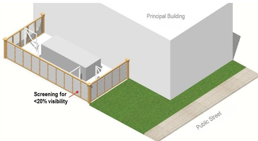
Figure 11-604(C). Ground Equipment Screening
